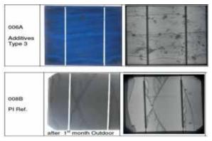
Figure 6. Different visual appearance of snail trails depending on additives in EVA [2]
