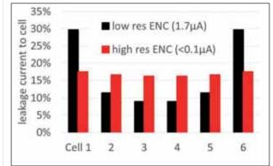
Figure 2. Leakage current distribution depending on kind of encapsulation material (high volume resistivity (10 <sup>15</sup>  $\Omega$ cm) versus low volume resistivity (10 <sup>13</sup>  $\Omega$ cm)) [1]
