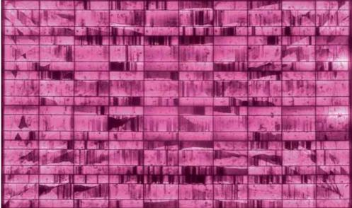
EL imaging from mobile testing highlights inactive cell areas in modules in the field
