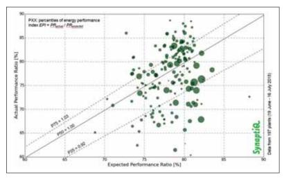
Figure 1: Actual performance ratio (PR) from monitoring versus expected PR based on plant specification and real weather data for 197 PV plants in Europe; the worst 25% perform more than 8% below expectation; the dot size represents the size of the PV plant
