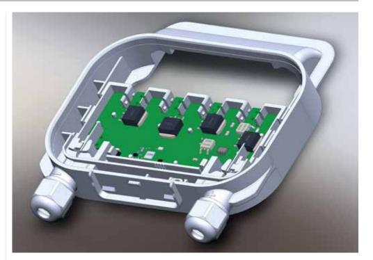
Platform: The SunSniffer sensor measures voltage and temperature at each single module, and the simulation engine in combination with artificial intelligence allows the system to detect even the smallest error - with an accuracy of under 1%, according to the company. The
