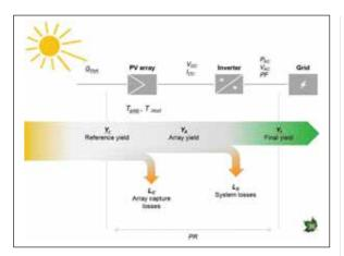
Figure 2: Energy flow in a grid-connected PV system; with measurements of plane-of-array irradiance (GPoA), DC voltage and current (VDC, IDC), AC power, voltage and power factor (PAC, VAC, PF), ambient and module temperature (Tamb, Tmod); yields (Y), losses (L) and performance ratio (PR)
