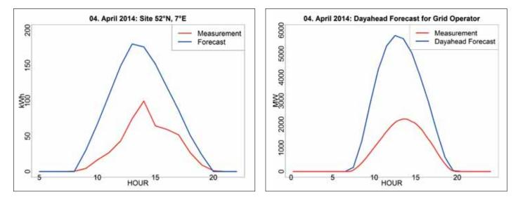
Figure 1. The difference between forecast and actual production during a Saharan dust outbreak for a single site (left) and at a grid level
