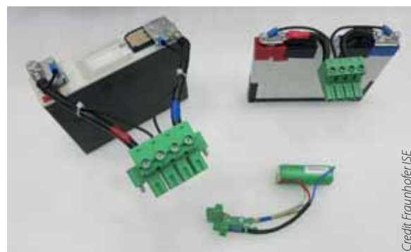
Figure 2. Lithium-ion cells used in home storage system prepared for test
