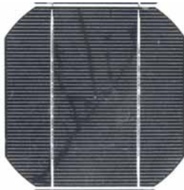
Figure 4. EL image and photograph of a solar cell affected from grid finger discoloration. The patterns of cell cracks and discoloured stripes are completely identical
