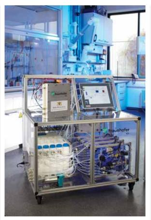
Figure 1. Kilowatt-class vanadium oxygen fuel cell system
