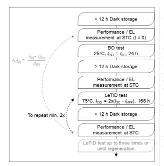
Figure 6. Test sequence of BO and LeTID test
