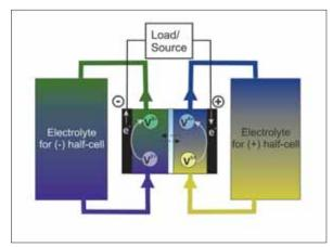
Figure 2. Schematics of vanadium redox flow batteries
