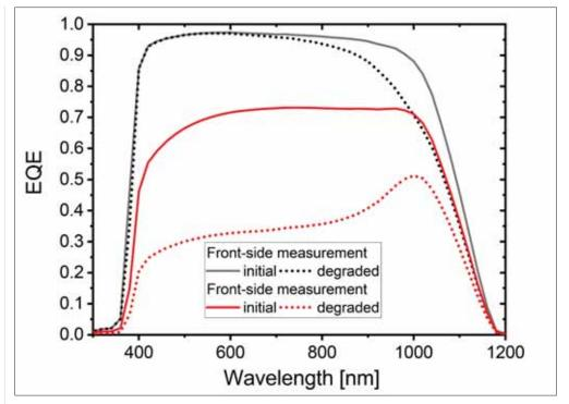
Figure 2. External quantum efficiency (EQE) of a bifacial PERC one-cell module. Compared with the initial state (solid lines), the measurements in the degraded state (dotted lines) have reduced EQE signals in certain wavelength ranges as a result of PID
