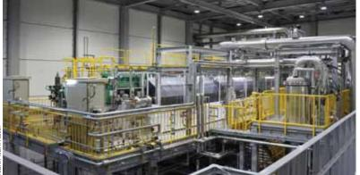
Alkaline-water electrolysis system by Asahi Kasei at the FH2R project in Fukushima, Japan
