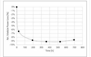
Figure 7. Module power loss due to BO and LeTID
