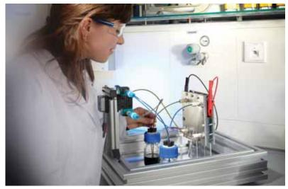
Figure 3. Vanadium redox flow laboratory test cell setup
