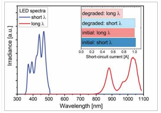
Figure 3. Two spectra of an LED solar simulator for rapid rear-side PID testing, representing the shortwavelength range (blue line) and the long-wavelength range (red line). The inlay shows the resulting shortcircuit current of a bifacial one-cell module for the two indicated spectra in the initial and degraded states. While there is almost no change in the current for the short-wavelength spectrum, the long-wavelength spectrum clearly shows the rear-side degradation
