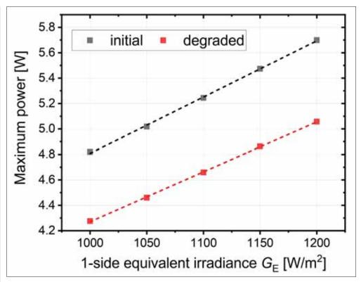
Figure 1. Power ( $P_{max}$ ) of a mini-module as a function of the one-side equivalent irradiance  $G_{F}$
