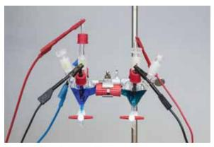
Figure 5. Discharged non-flow vanadium redox flow battery laboratory cell
