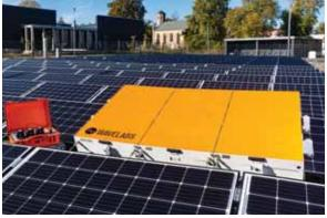
Figure 4. LED-based solar simulator at the Fraunhofer CSP bifacial PV park. Using different coloured LEDs, an initial diagnosis of the type of PID can be made
