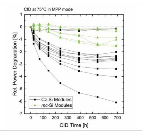
Figure 4. Results of LeTID benchmark showing the power degradation of commercial modules during LeTID test at 75°C and  $I_{co} = 1.0A$ . Figure adapted from [17]
