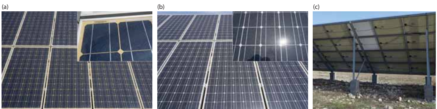
Figure 2. Four-year-old field modules with: (a) a single-sided PVDF backsheet (Ningxia); (b) a PVF backsheet (Ningxia); (c) a PET backsheet (Inner Mongolia)
