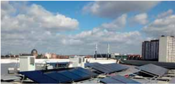
Figure 1. Test site measuring illumination, temperature, wind, and energy output with one-second resolution
