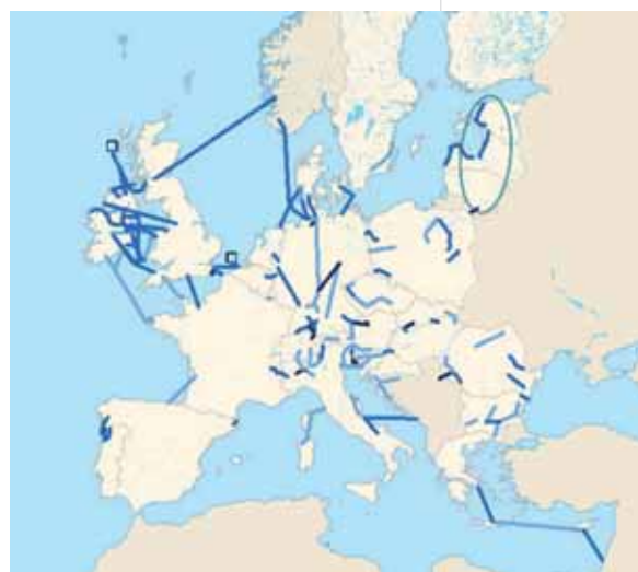
Existing (dark blue) high-voltage lines, those planned for completion pre-2020 (mid-blue) and those planned for after 2020 (pale blue). Adapted from Platts and European Commission data
