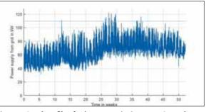
Figure 7. Load profile of a data centre in Germany. Annual savings of more than €1,000 can be realised if the peak demand is reduced by 12kW (blue line)
