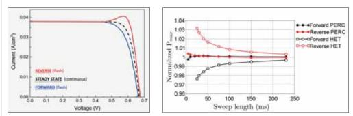
Figure 2. Left: IV curves for forward (blue) and reverse (red) short pulse sweeps compared to a steady-state IV measurement. Right: P<sub>mx</sub> performance measurement for PERC and SHJ modules as a function of pulse length on an Eternalsun Spire long-pulse solar simulator. Measurements converge at pulse lengths above 200ms, not attainable for conventional flash solar simulators
