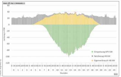
During summer, the APV system covers the electricity load at the farm almost completely. The green area represents the feed-in of the solar power into the grid, the yellow area represents the own consumption, while the purchased power from the grid is plotted in grey
