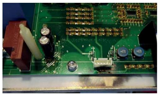
Figure 4. Delamination and internal corrosion in an inverter following passive chamber testing
