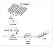
Figure 2. Simple PV system block diagram
