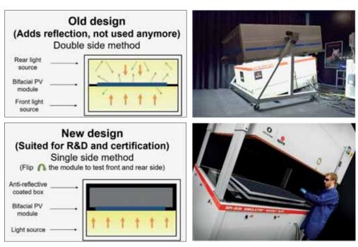
Figure 8. Two bifacial characterisation methods of bifacial with reduced footprint, tested by Eternalsun Spire. The single-side setup is commercially available and already installed around the world
