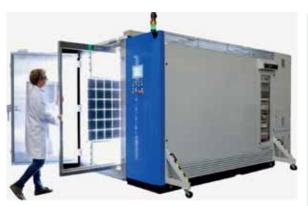
Figure 10. Climate Chamber Solar Simulator (CCSS), capable of performing accelerated temperature, irradiance and humidity test on modules of different PV technologies
