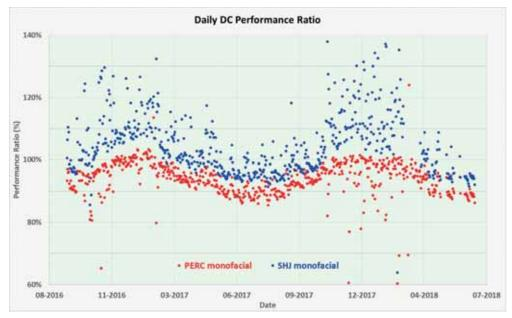
Figure 12. Outdoor monitoring of the average daily system performance ratio over the years 2016-2018 at the site of CEA-INES in Bourget-du-Lac (France). Monofacial PERC modules in red, monofacial SHJ modules in blue
