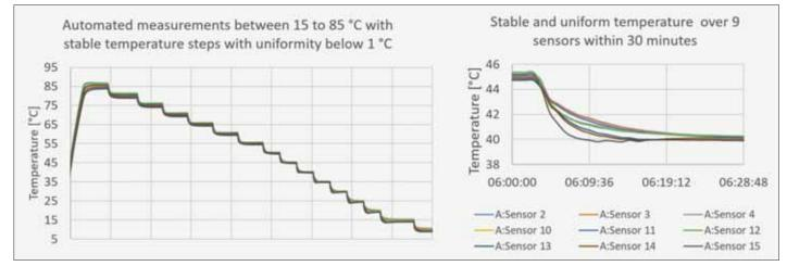
Figure 6. Temperature of the PV module on nine points across the module versus time during the P<sub>MAX</sub> versus temperature test shown in Figure 5. Note that the temperature is stabilised for accurate P<sub>MAX</sub> measurements. Test performed on the Eternalsun Spire setup shown in Figure 3
