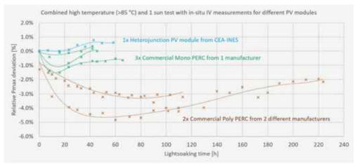
Figure 11. In-situ LETID testing on PERC modules from different manufacturers, showing up to 5% degradation and subsequent regeneration to different extents; and on a heterojunction PV module from CEA-INES, which does not show any degradation but a regeneration of about 1%
