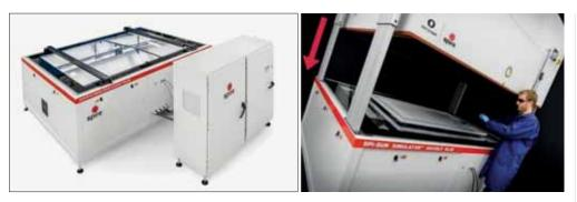
Figure 3. Left: SPI-SUN 5600 SLP table top simulator from Eternalsun Spire. Right: the same setup with an added temperature control box on top, ready for single-sided bifacial measurements
