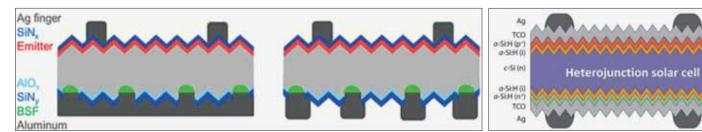
Figure 7. Layout of monofacial PERC (left) and bifacial PERC+ cell (middle) and heterojunction cell (right)
