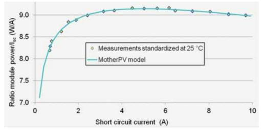
Figure 9. Mother-PV method: measurement and modelling of the ratio of  $P_{Max}/I_{sc}$  versus  $I_{sc}$  (at 25°C). Plotted against the short circuit current  $I_{sc}$  that serves as a self-reference for irradiance
