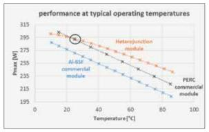
Figure 5.  $P_{max}$  under one sun versus temperature for SHJ, PERC and Al-BSF modules measured on Eternalsun Spire labflasher with temperature box. The black circle points to the performance of SHJ and PERC at STC conditions (25°C)
