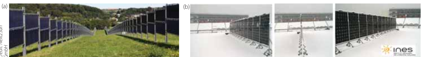
Figure 4. (a) vertical bifacial configuration for agri-voltaics (left); (b) vertical test bench with bifacial heterojunction modules during winter at CEA-INES (Bourget-du-Lac, France)
