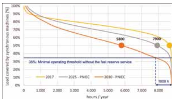
Figure 9. Current and future load coverage by synchronous machines in Italy. Source: Terna
