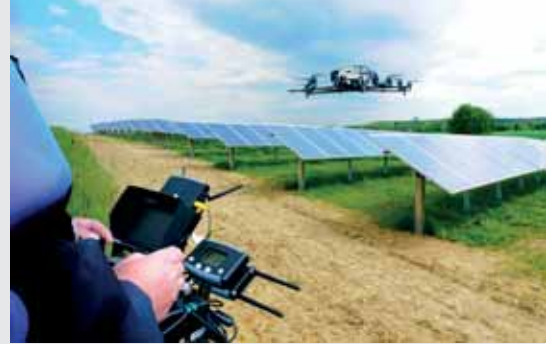
Drones can be used for visual and thermographic inspections of a plant during commissioning.
