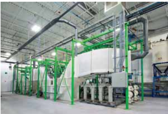
Figure 7. First Solar's third-generation PV recycling technology based on a continuous-flow process
