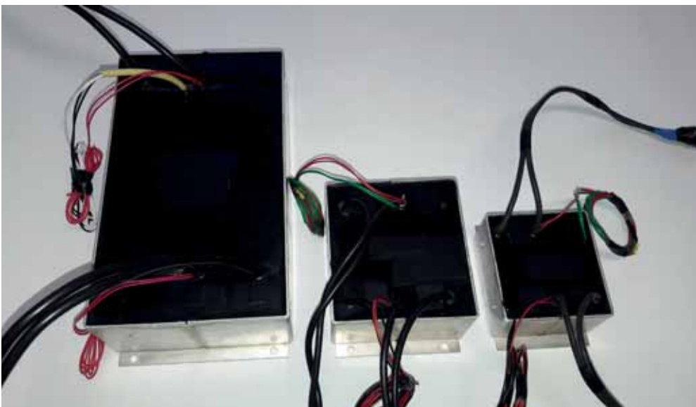
Figure 1. Example of weight/volume reduction of inductors
