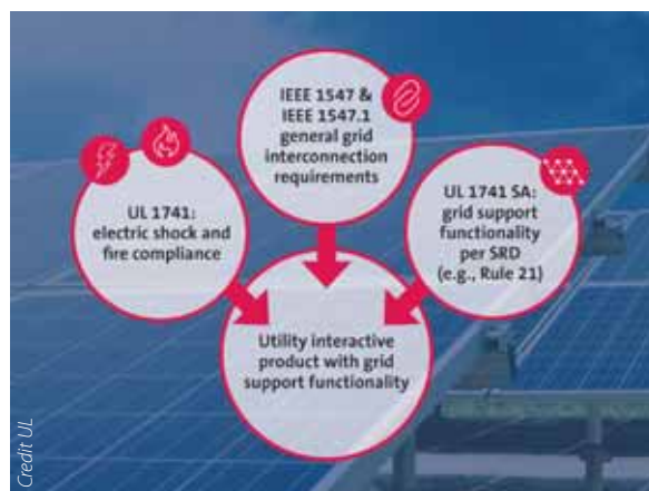
Figure 2. The standards used to evaluate a utility-interconnected product with grid support capabilities
