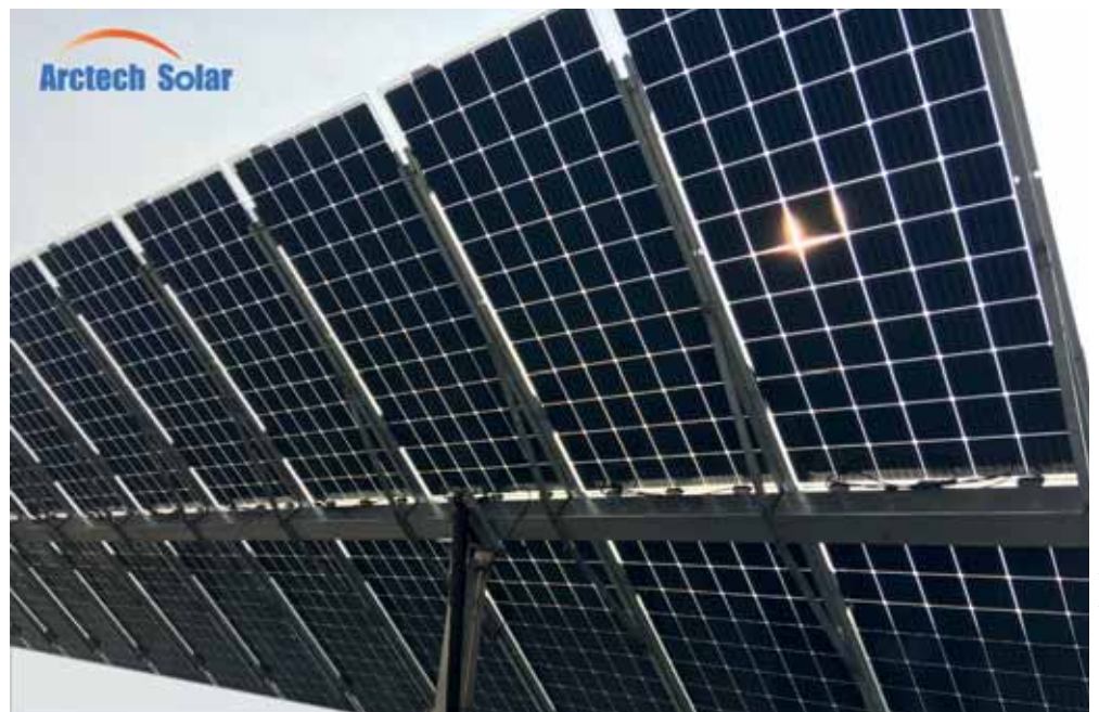
Figure 3. Independent horizontal single-axis tracker from Arctech Solar, designed for bifacial modules [145]. The modules are fixed using aluminium elements at the module edges, overlapping with the long purlins to avoid covering the back of the bifacial modules. Junction boxes at the module edges in such a system, as shown, can be integrated without shading caused by cables.
