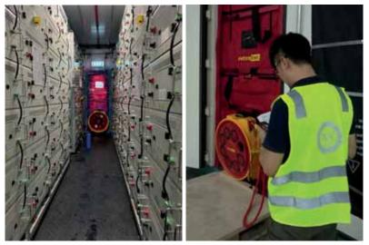
Figure 7. On-site testing of "enclosure integrity" of door fan as required by NFPA 2001 regulation (USA: National Fire Protection Association: Clean Agent Fire Extinguishing Systems)
