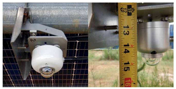
Figure 4. Rear-side pyranometer mount. Options for rear-side pyranometer mounting systems are currently limited and non-standard. Most mounting systems will result in the pyranometer being some distance away from the back of the modules
