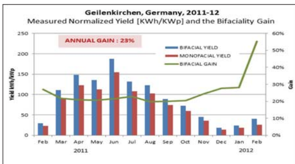
Figure 11. Monthly energy gain of a bifacial versus a monofacial PV system
