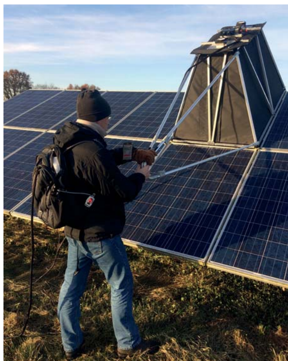
Figure 1. Fluorescence outdoor inspection system (FLOIS) in operation on a PV generator
